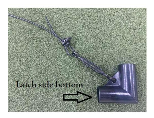
Connect the cable through the other corner in the same way, only without a turnbuckle (cable through clamp, then through corner and back into clamp then tighten)
